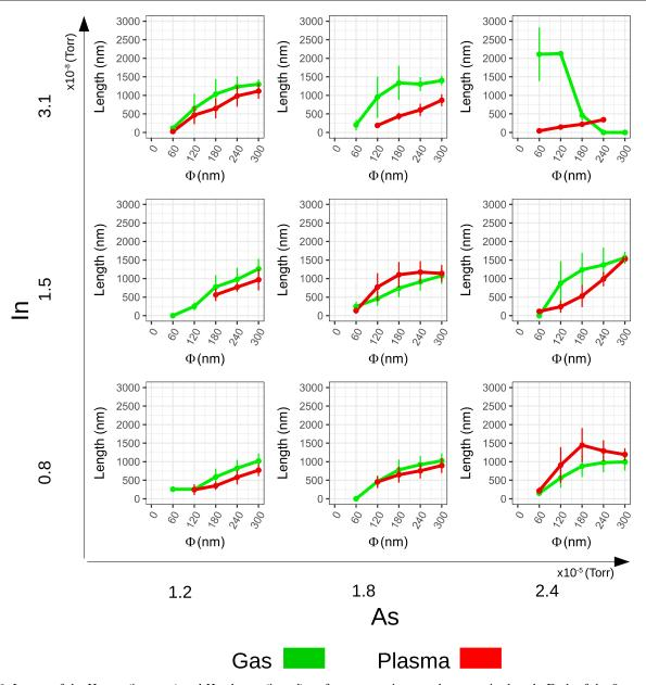
**Figure 3.** Impact of the  $H_2$ -gas (in green) and  $H_2$ -plasma (in red) surface preparations on the nanowire length. Each of the 9 scatter plots correspond to different growth conditions (In and As fluxes reported on left and bottom, respectively). For each plot, the *x*-axis corresponds to the diameter (in nm) and the *y*-axis to the length (in nm) of the corresponding nanowire family. Green lines correspond to a  $H_2$  gas preparation, whereas it is  $H_2$  plasma for the red ones.
