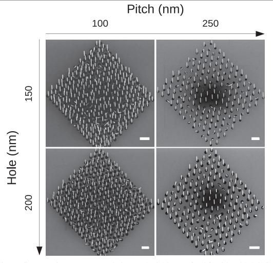
**Figure 5.** SEM images of InAs nanowires grown on patterned substrates. The pitch increases from left to right and the hole diameter from top to bottom. The Indium flux is  $6.2 \times 10^{-8}$  Torr and the Arsenic one is  $0.6 \times 10^{-5}$  Torr. Scale bars are 500 nm.
