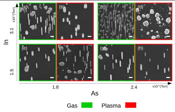
**Figure 1.** Evolution of InAs nanowire morphology as a function of growth conditions and surface preparation. The In flux increases from bottom to top and the As one from left to right. The green framed SEM images (a), (c), (e), (g) correspond to a  $H_2$  gas surface preparation whereas it is a plasma one for the red frames (b), (d), (f), (h). The scale bar is 500 nm.
