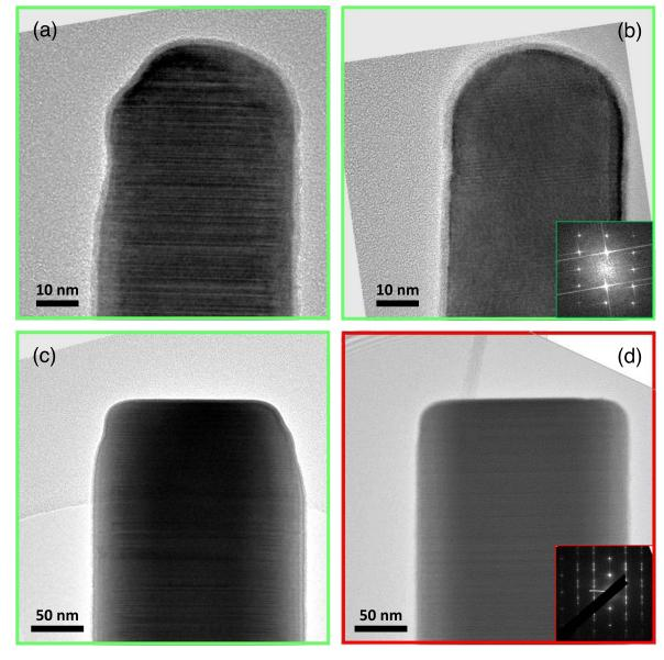
**Figure 4.** Flat and rounded shapes of the InAs nanowire tips viewed by HR-TEM. (a), (b) correspond to an InAs nanowire from figures 1(c). (c), (d) correspond to figures 1(e), (f), respectively. (a), (c) and (d) are viewed along the [110] direction, while (b) is viewed along the [112] direction (rotation of  $30^{\circ}$ ). The growth direction is <111> in all the cases.
