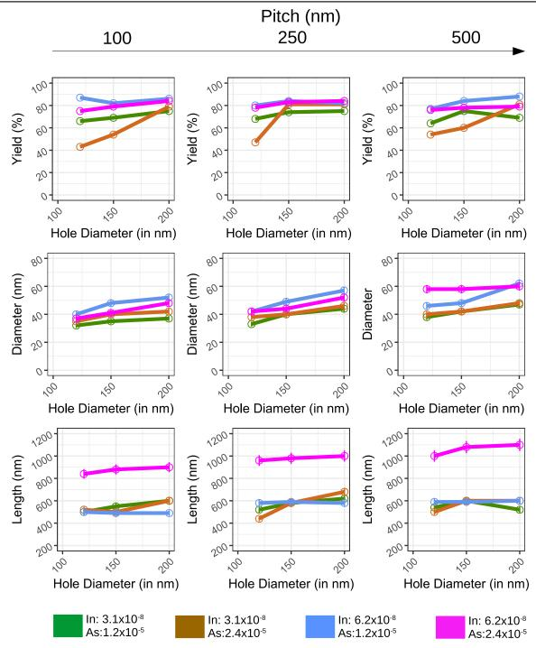
**Figure 6.** Statistical analysis of the InAs nanowire grown on patterned Si(111) wafers. Each color corresponds to a specific set of growth conditions: (i.e. a specific In and As flux). For each plot, the *x*-axis corresponds to the pattern hole diameters (in nm). The *y*-axis represents the vertical yield (in %) for the 1st line, the mean diameter (in nm) for the 2nd line and the mean length (in nm) for the 3rd line. Each column corresponds to a different pitch: 100, 250 and 500 nm.
